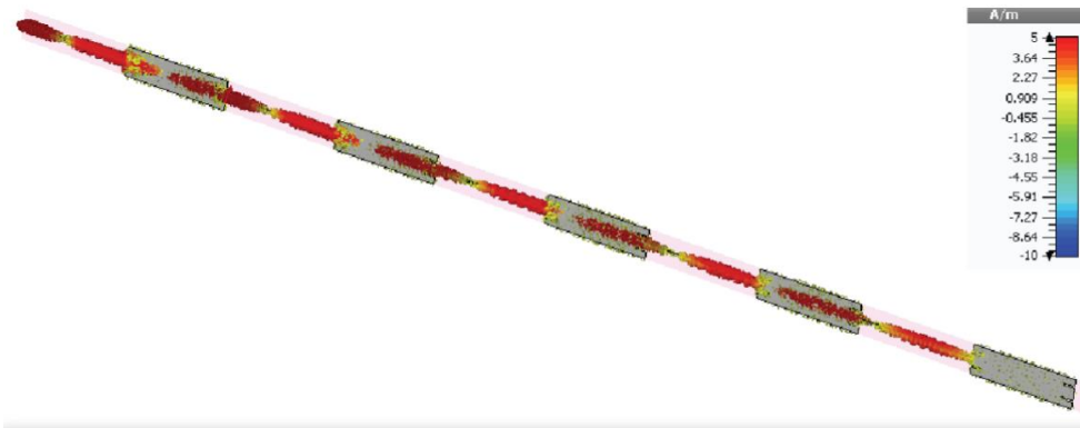
Figure 4. Simulated current distribution of the proposed antenna at frequency 1.1GHz.
